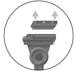
**Attach Camera Mounting Shoe** to the RCMB bracket using the mounting hardware.
